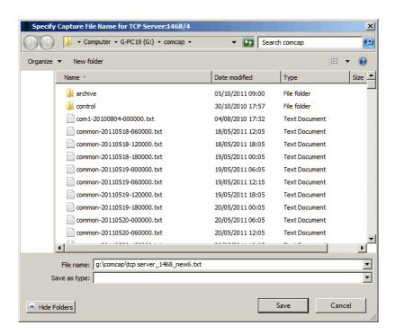
Note that capture will not start until the file name is specified. An existing file name may be used, with captured data added to the end of the file. This feature is intended for applications where data is being captured from a single device for a specific purpose, such as a laboratory test. The 'Add Comment to Log' right menu option might also be useful to add information to the capture log.
