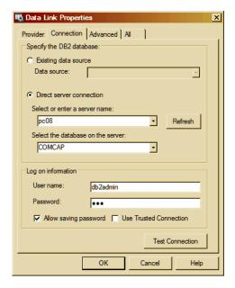
On the Connection tab, choose 'Direct Server Connection' with the server name as an IP address or host, it should then allow a database to be selected once a logon has been entered and 'Allow Saving Password' ticked. Click Test Connection to make sure SQL is working, then OK.
