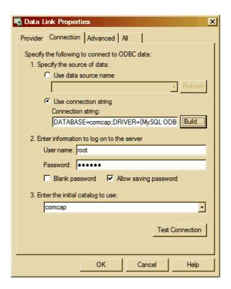
Specify authentication to logon to the database, and then the actual database to be used. Click Test Connection to make sure SQL is working, then OK
