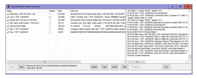
The main ComGen window shows data generation channels in the left pane, and log on the right. There are buttons to Start and Stop data generation, to hide the window and to access the Settings window.
