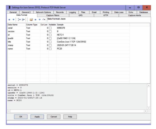
Specifying the data formats Json and XML is the same as 'variable named columns'. The sample data is parsed to separate the data names from the data values. Any named columns not found are treated as blank or null.
