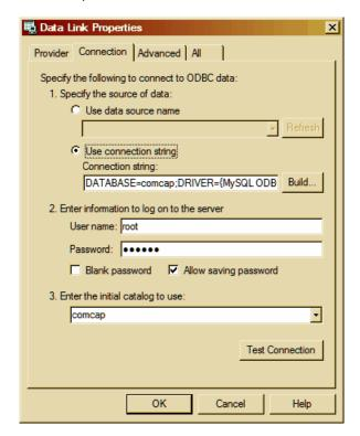
On the Connection tab, choose Use Connection String and click the Build button. A Select Data Source dialog will appear (shown below) from which an existing ODBC connection for MySQL may be chosen, or the New button clicked to create a new data source:
