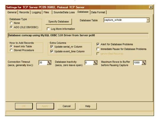
ComCap will then open the database and the details will be displayed to confirm it's all working OK. ComCap can either insert data directly into a table, or pass data to a stored procedure that may
