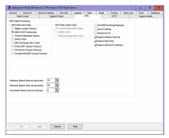
If GPS Data Processing is specified for this channel in Common Settings, Network Channels or Common Settings, Network Channels, these settings define how GPS data should be processed.
