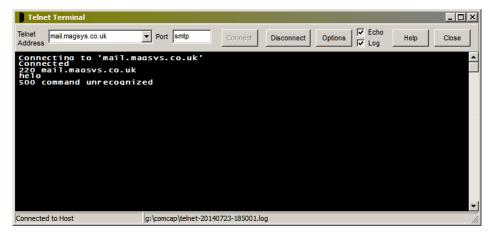
This window provides ANSI terminal emulation using the TCP/IP Telnet protocol to interact with a remote terminal server or host computer. The window is resizable depending upon desired size and screen resolution. A number of terminal options are specified through a dialog box. A log of each Telnet session may be saved, written to the normal logging directory with a file name format telnet-yyyymmdd-hhnnss.
