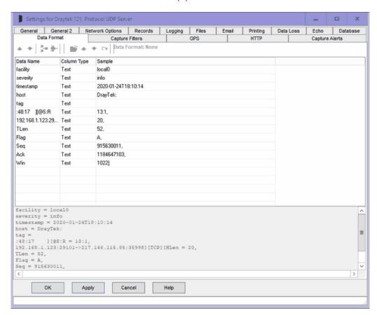
Specifying the data format 'variable named columns' is similar, except the data column name is specified instead of the sequence. The sample data is parsed to separate the data names from the data values. Note spaces are not allowed in the data names. Any named columns not found are treated as blank or null.
