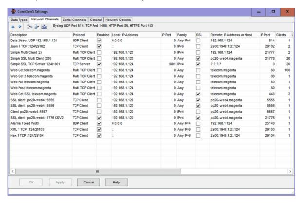
Network configuration is very similar to Common Settings, Network Channels, Local and Remote IP and Port at the same. To simplify this grid, retry attempts have been made common to all channels and are specified on the Network Options tab, see below. Note that SSL is set-up in the grid, unlike in ComCap4. A remote host name can only be specified if Family Protocols are slightly different.
