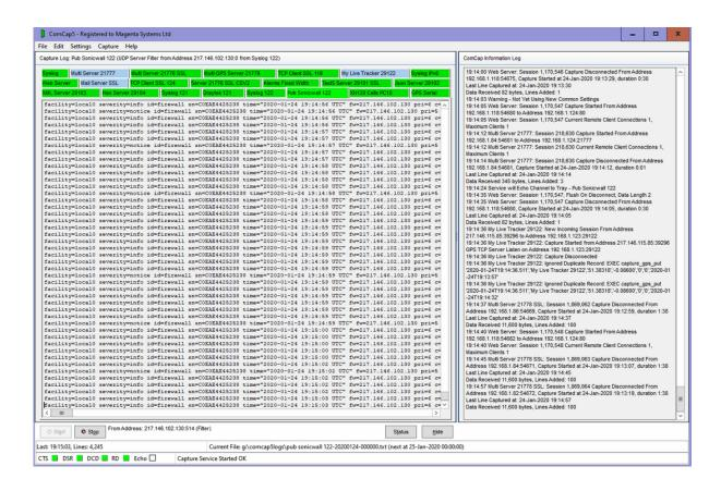
The example here has numerous test channels set-up and running, green tabs means OK, red would be not running. A new install will not have any tab.
