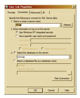
On the Connection tab, select or enter a SQL server name (it may be available in the drop down box, but may need a UNC path or IP address entered), then specify authentication to logon to the database, and finally the actual database to be used. Click Test Connection to make sure SQL is working, then OK.
